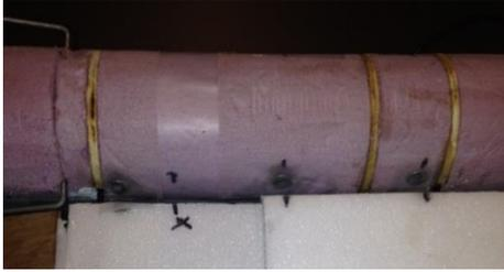
**Figure 19:** Wing Connection to Fuselage.
