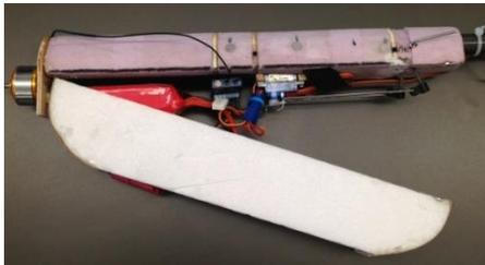
**Figure 20:** Hatch Partially Detached from Fuselage.
