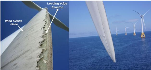
Figure 1: Example of leading edge erosion and no damage
