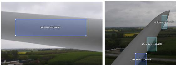
Figure 2: Examples of manually annotated damages related to wind turbine blades
