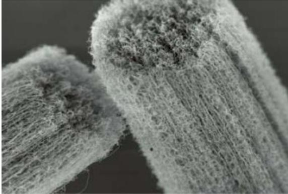
Figure 3: Scanning electron microscopy image of carbon nanotube bundles [8]
