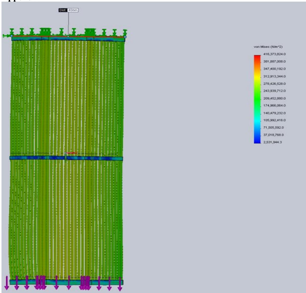
*Figure 7: The Standard Model is under stress with the blue epoxy composite ribs experiencing less stress. The purple arrows are loads attached to the model, while green arrows are fixed points on the model. As per the metric on the right of the image, blue regions experience less stress than green region.*
