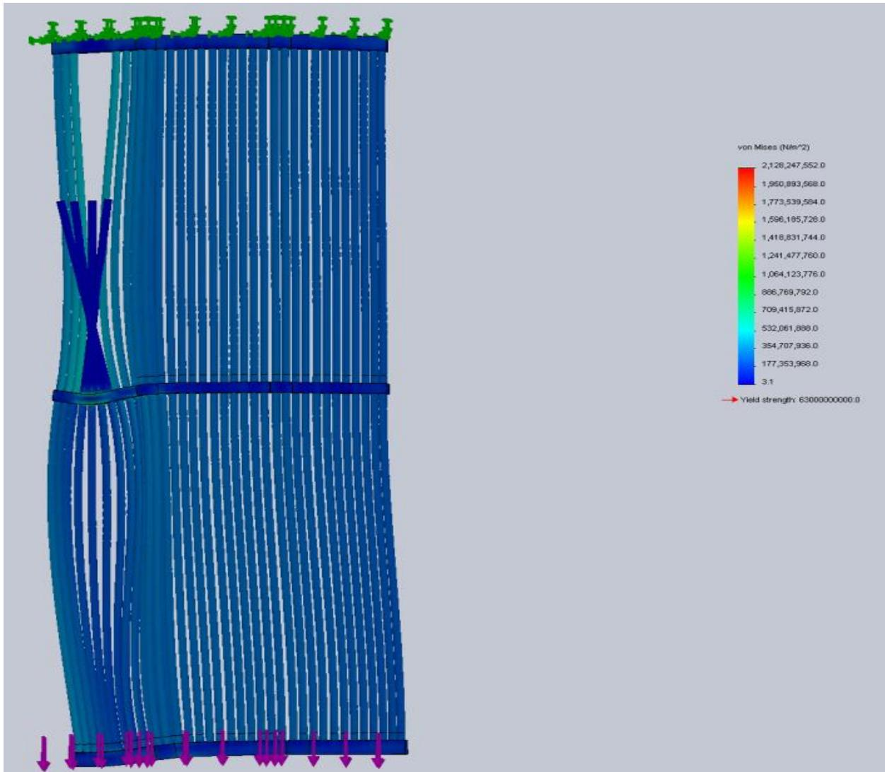
Figure 8: The damaged Standard Model design has a large hole in it to mimic performance after meteor damage. While it looks blue, the colors on the metric correspond to different values as those in Figure 7.
