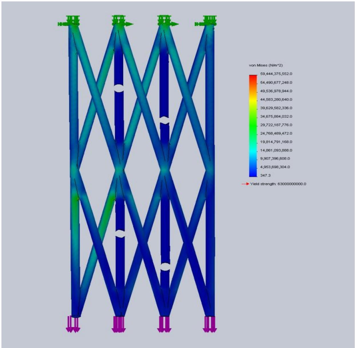
Figure 10: The “damaged” Hoytether Model, with holes to mimic performance after meteor damage.
