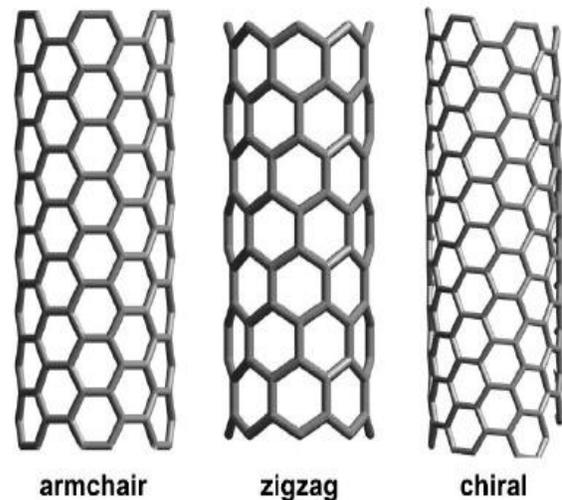
*Figure 2: Carbon nanotube microstructure designs [6]*
