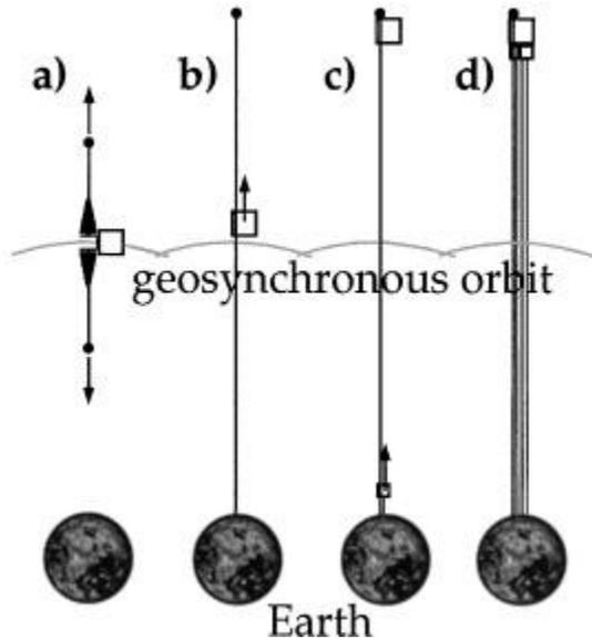
Figure 1: Earth and space elevator combination showing increasing cable thickness [3]
