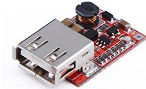
Fig. 8 USB charging circuit
