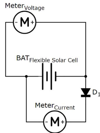
Fig. 4 Circuit configuration of solar cell in series with diode
