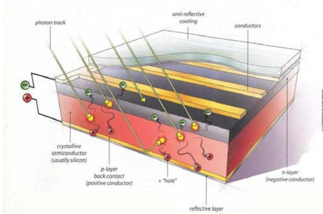
Fig. 1 Diagram of photovoltaic cell
