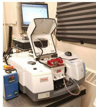
Fig. 2 FTIR spectrometer used in Rutgers University's Chemical and Biochemical Engineering Department.
