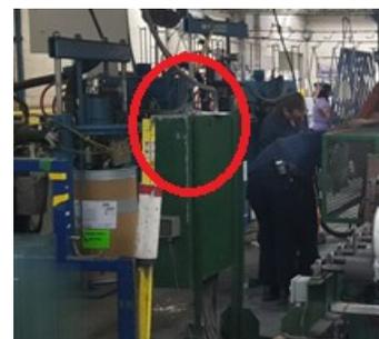
Fig. 5 Electronic box was a possible location for the andon light
