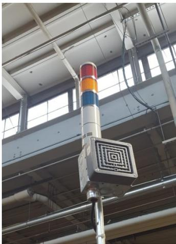
Fig. 9 Speaker on the andon light system of the vertical line plays a loud tone to alert mechanics when there is a problem
