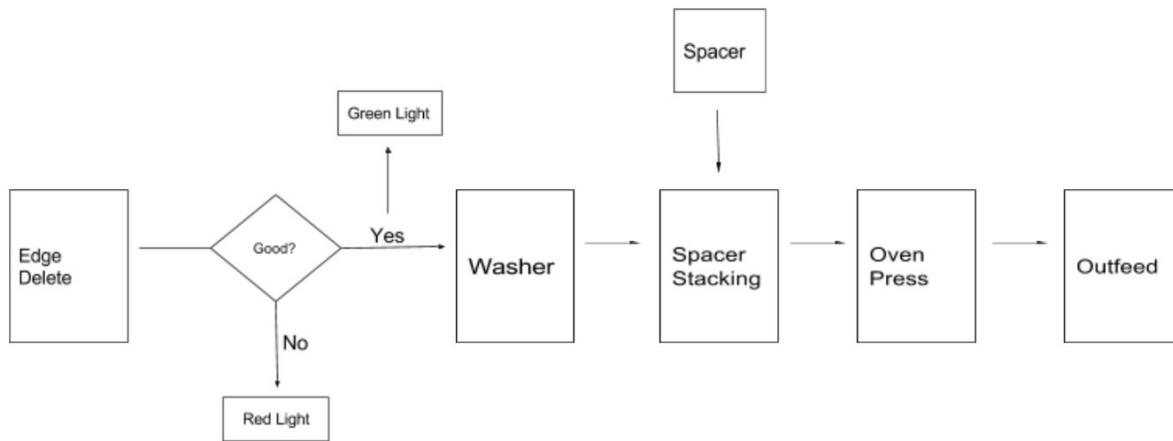
Fig. 3 Process map of glass intercept line detailing current quality check system
