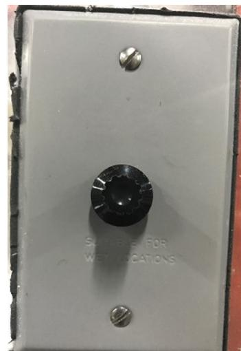
Fig. 10 Dial for the andon lights currently installed on the extrusion line
