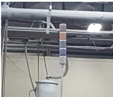
Fig. 1 Andon light on the extrusion line
