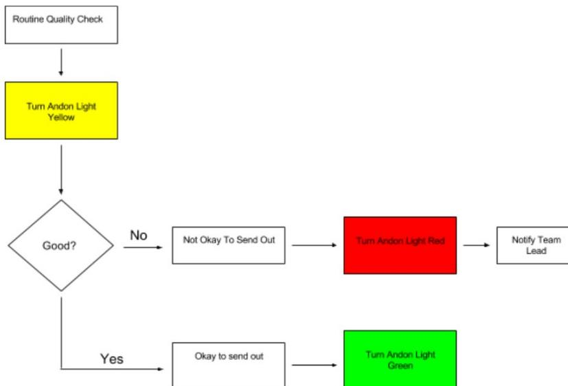
Fig. 8 Andon light procedure to guide employees when and how to use the andon light
