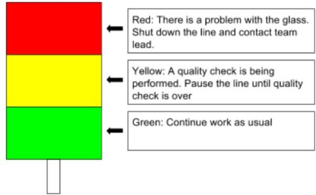
Fig. 12 Andon light system instructions created to guide worker once the quality check is implemented
