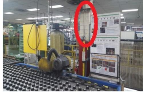
Fig. 4 Column in front of edge delete station was a possible location for the andon light
