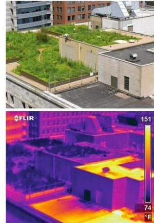
Fig. 1 Thermal imaging exhibiting temperature difference of two adjacent roofs with and without vegetation [7].
