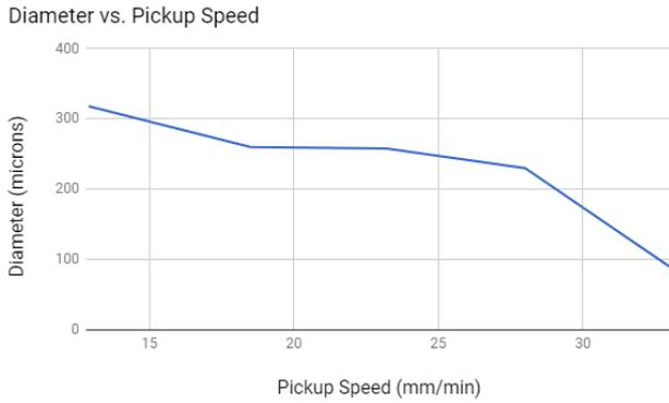
Figure 8 Extrusion Results
