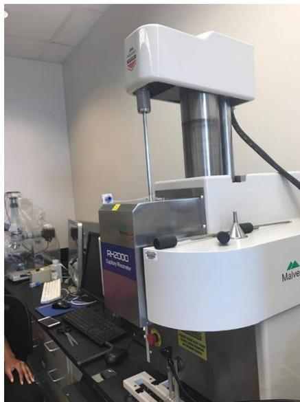
Figure 7 Extruder: RH2000 Capillary Rheometer
