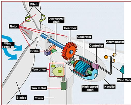
Fig. 1: Diagram of HAWT [10]
