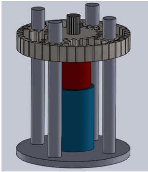
Fig. 3: Planetary Gear Mechanism
