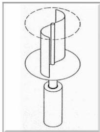
Fig. 9: VAWT with Savonius design [16]
